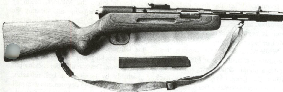
Two large holes in the Bergmann's magazine well serve to lighten this heavy gun.
