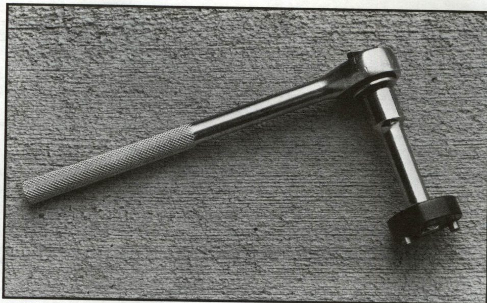
Tom Seslar's ingenious disassembly spanner snaps onto a standard 3/8-inch socket wrench. Photo by Al Paulson.
