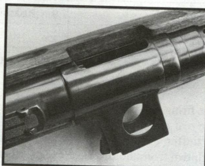
Two large holes in the Bergmann's magazine well serve to lighten this heavy gun.
